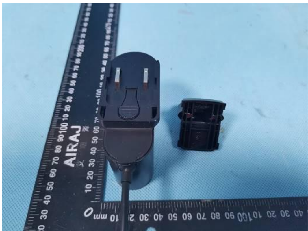
Figure 2 Overview of unit with detachable EU plug
