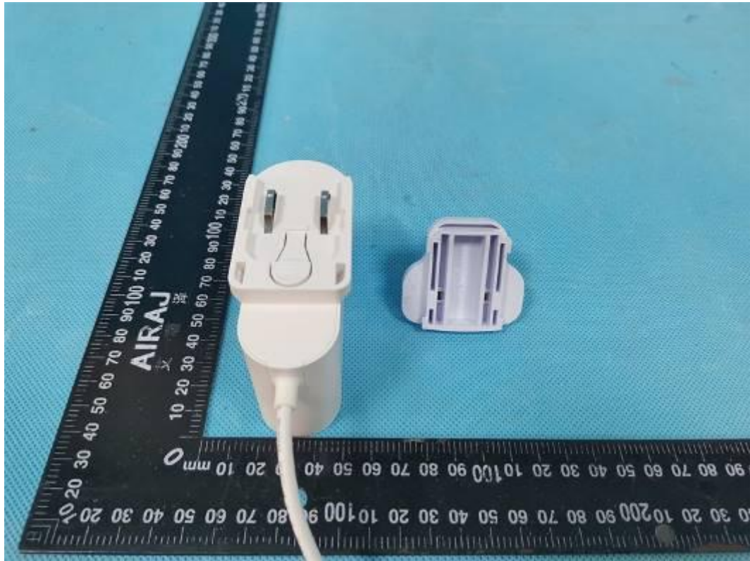
Figure 7 Overview of unit with detachable UK plug
