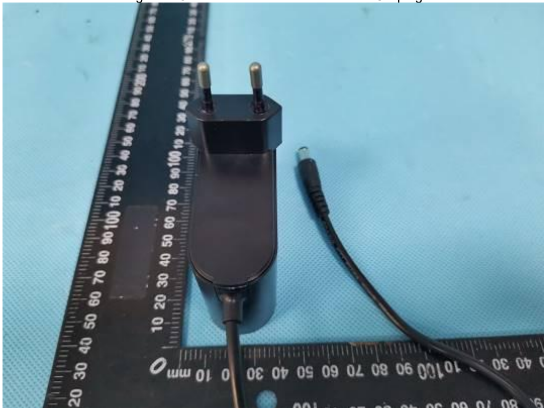
Figure 8 Overview of unit with fixed EU plug
